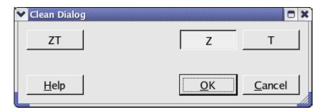
Click component toggle buttons required to be cleaned. Click OK button to perform the cleaning, or Cancel - to close the window without cleaning.
