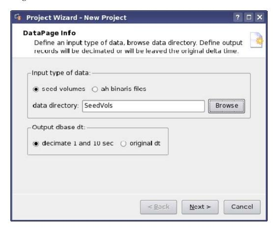
Select the type of data in *Input type of data* frame. The radio button *seed volumes* - the data base will be created from seed volumes. The radio button *ah binaries files* - the data base will be created from AH binary files.
