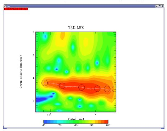
To make a floating filtering it is necessary to plot dispersion curve to make phase equalization (black circles). Use mouse to do this. Click left mouse button to put a point and the right one to delete the point nearest to cursor location. Type "e" to finish the plotting.
