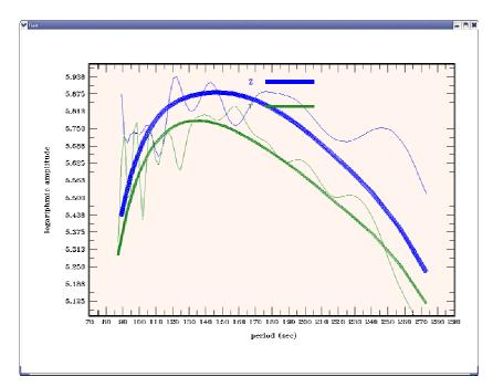
Thin lines present the amplitude spectra of raw signals; thick lines present the amplitude spectra of cleaned signals.
