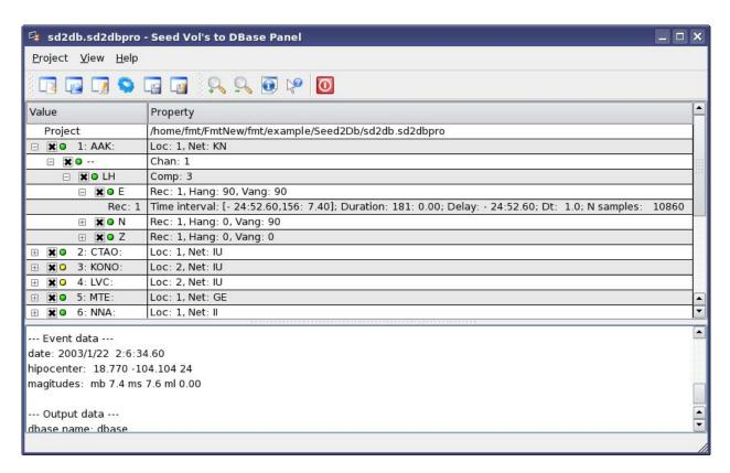
DbCreator is a program for creating Data base of seismograms for further processing by Frequency time analysis program. It's interface is a C++ code using Qt C++ tool kit for multiplatform Graphic User Interface and application development. The computational part of program is based on Data Base package of programs designed by Daniel Quinlan (IRIS corporation).
