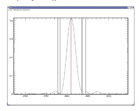
It is necessary to cut a signal which you've selected. This signal is concentrated near the center of picture (red vertical line). To do this you must set four points to define the filtering window with cosine edges. Use the same commands as above.
